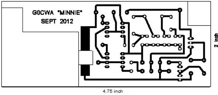
You may notice that D1, D2, C11 and C12 do not appear on the PCB top they are actually soldered on the underside of the board to save space. There are also two wire links on the top of the PCB to add.
