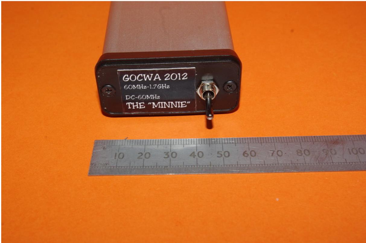
There is nothing clever or particularly original in the design with one exception the use of a 125MHz conversion oscillator so avoiding the VHF broadcast band on the output and reducing any sensitivity issues. The 5V supply is taken off the dongles USB connector by opening up the dongle case, carefully, and soldering a fine insulated wire to the appropriate USB connector pin taking this out through a small opening cut in the side of the dongle case.
