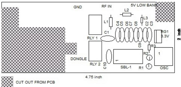
The coils are all 6.5 turns of ~1mm diameter copper wire 0.25 inch diameter by 0.4 inch long, the relays are both NEC/TOKIN UB2-5NE 5V Coil DP Ch-over types although any similar equivalent ones may be used. The regulator is an LM1117T 3.3V unit. The crystal oscillator is a 3.3V 125MHz crystal oscillator module, any oscillator module frequency above 60MHz can be used but I can't guarantee the receivers performance or immunity to de-sensitisation/interference from the VHF broadcast bands.
