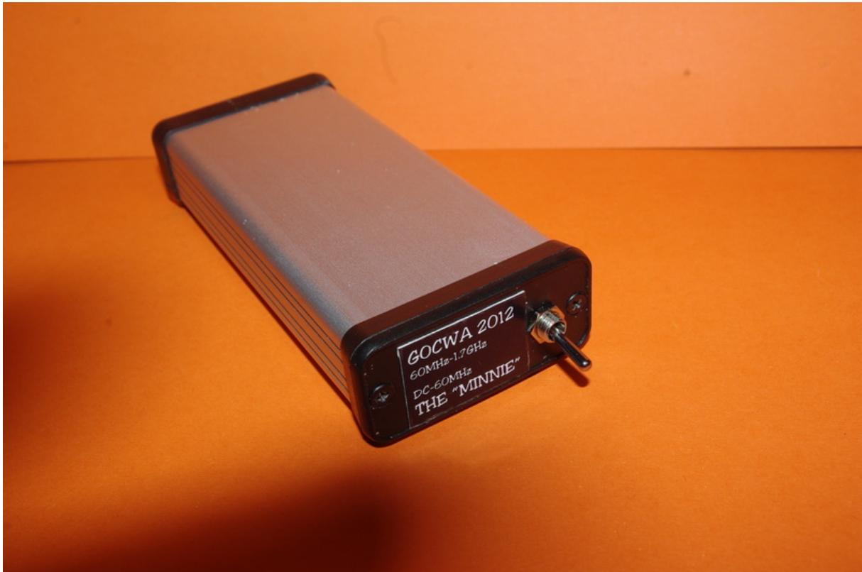
Hi this is my latest design for a RTL-SDR communications receiver. The set amounts to little more than a switchable receive up converter. Although designed for the Realtek RTL2832U Chipset + Elonics E4000 tuner, it will work with any of the other compatible tuners. I would personally recommend SDR# as the control package for the dongle.
