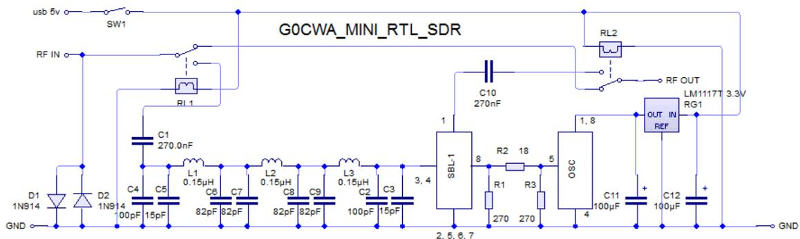
Follow my track layout and use top quality miniature co-ax for maximum sensitivity I used silver plated. Do NOT use single strand wire for any RF signals as these dongles are very sensitive to mismatches and unless you are very lucky will shut down and work poorly, if at all. Note I have presented the track layout as an X-ray view, remember to mirror it if needed for the copper side
