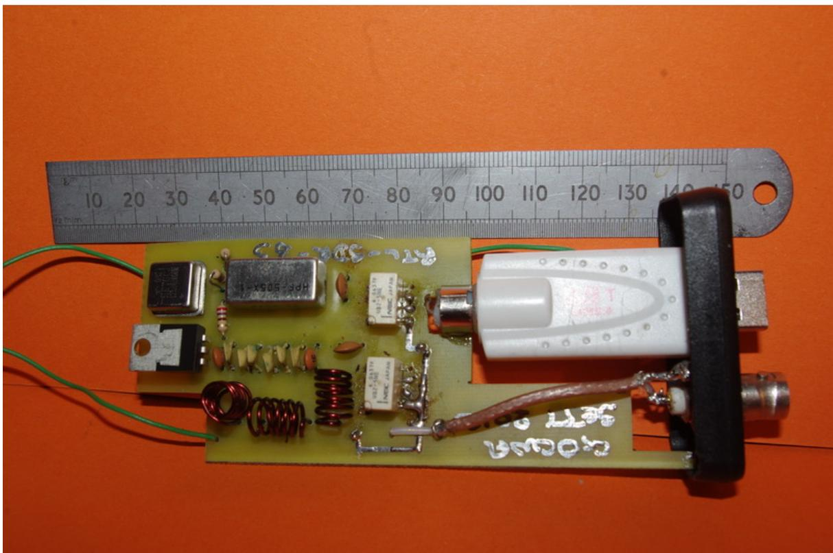
The RF input to the dongle is via a connector shown in the “real world” PCB layout diagram above. This connector was “scavenged” from a cheap plastic bodied co-ax plug which is soldered to the PCB in a small slot. TAKE NOTE the connector is soldered on both sides bridging the two earth pads to complete the ground track to both sides of the PCB; the centre pin is connected via a small piece of copper wire to the PCB.
